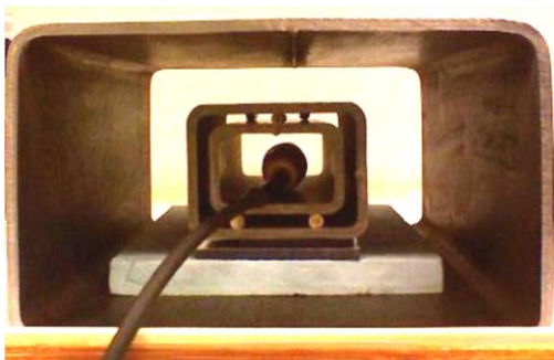
Fig. 1. The three layers of magnetic shielding. The Narda EFA-300’s MF probe is in place of the culture vessel. MF coils for exposure are below, but not in contact with the two smaller shields, insulated from the outer shield by a layer of rigid foam.
